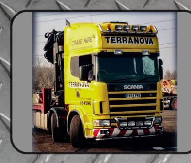
Scania with Hiab XS 600, a 16te hiab with remote control and four hydraulic out riggers.
