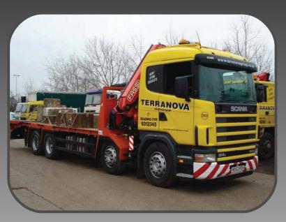
This vehicle is fitted with a FASSI F310AXP.24 with remote control and four hydraulic in/out outrigger legs, four extensions and hook application.
