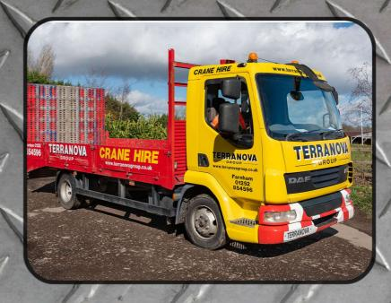
DAF LF45.140 - 7.5 tonne flat bed with tilted rear and loading ramp. Ideal for transporting light plant equipment.
