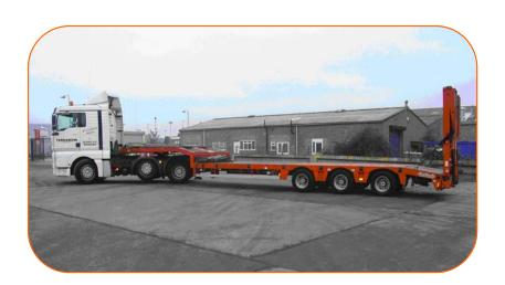
3 axel semi with fold down ramp.
