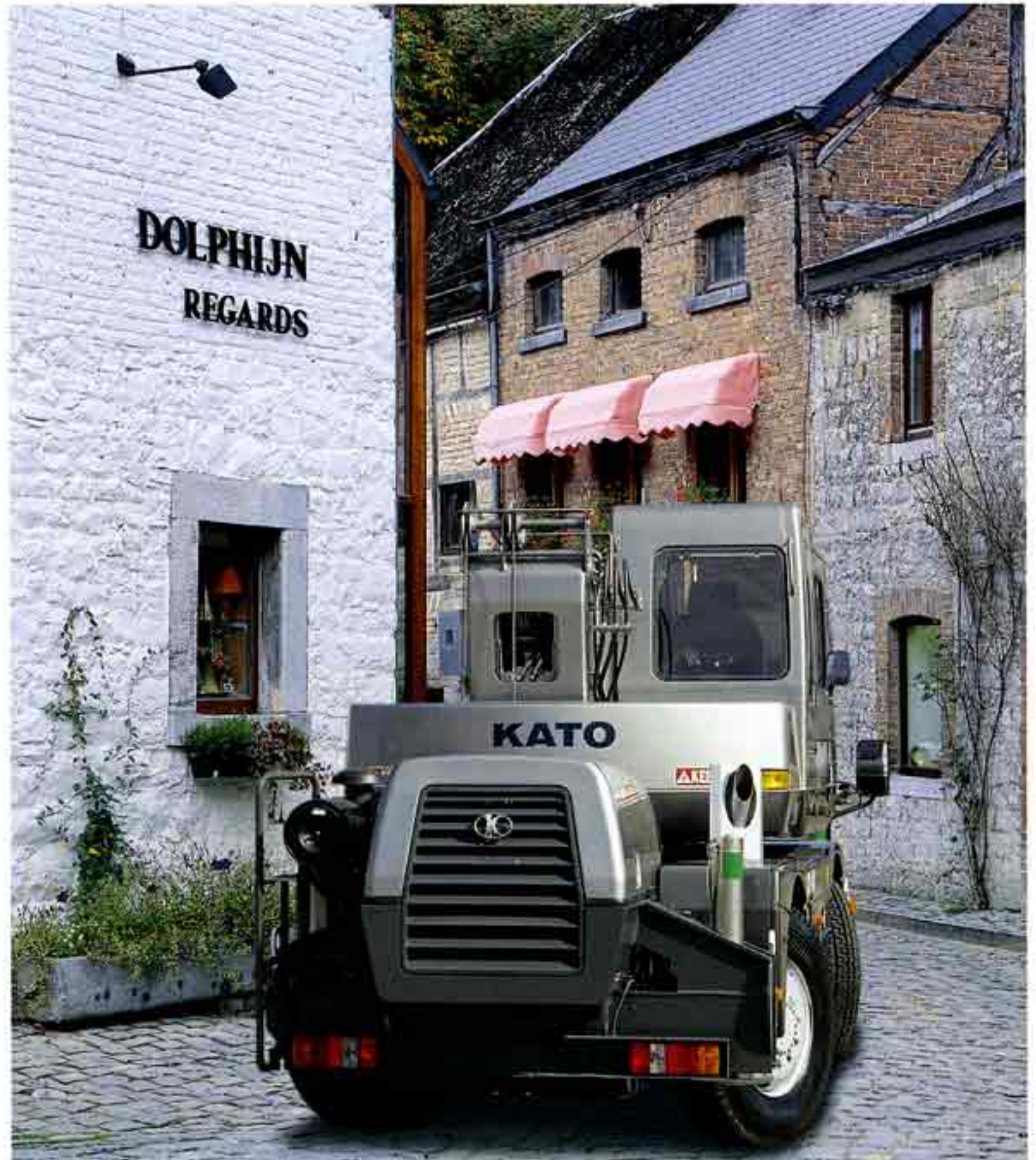
Minimum turning radius (Centre of extreme outer tyre) 3.92m (4 wheel steer) / 6.5m (2 wheel steer)
