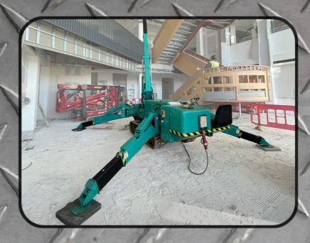
A compact 2.98t Minicrane with a 12.5m main boom. Designed for versatility and to work in all kinds of places. Easily manoeuvring on its rubber tracks within buildings. The 2 speed winch can reach loads 64m below the boom.
