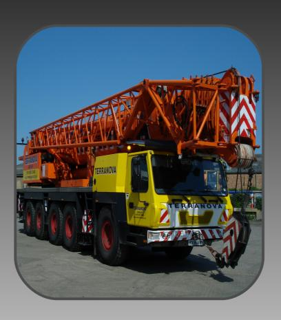
A compact 220t Crane With 68m main boom
