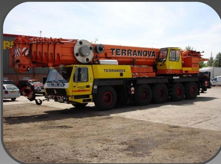
A 180t All Terrain Crane with 60 Metres Main Boom, 22 Metres Fly-jib And 63t cwt. Giving a lift capacity of 3.4t at 56 Metres radius
