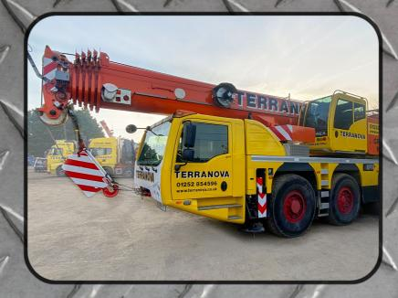
The Terex Challenger 3160 is a very light and compact 6 wheeled all terrain crane. It has an impressive lifting power for a vehicle with a turning circle of only 9m, a length of only 11.5m and extending boom with a native reach of 50m.
