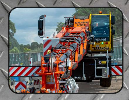
The Demag AC45 is a midrange City Class crane with all terrain abilities. Its all wheel steering and short base gives it outstanding manoeuvrability, yet its outriggers practically treble its pivot point along its length providing great stability.
